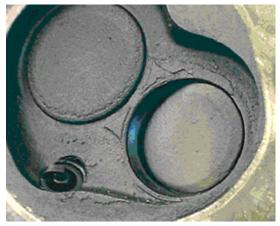
Valve seat recession generally affect the exhaust valve in the head. This is because this is the valve that opens to expel the burnt combustion gas. Inlet valves are lubricated by the petrol fuel mixture or only have air passing by them and hence are closed during and after combustion. Exhaust valve recessed into the cylinder head
